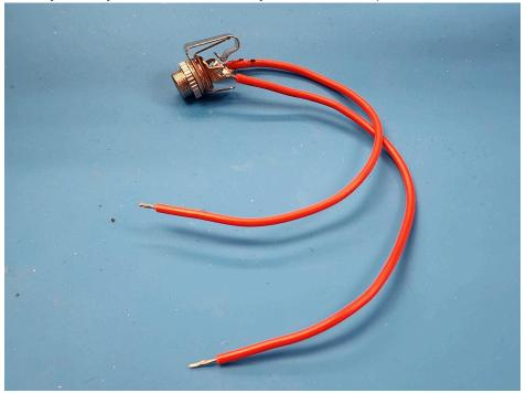
4. Twist together and solder each of the 2 free ends to each of the yellow wires that you cut in step 2.
