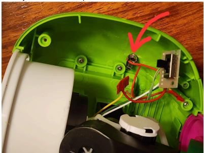
7. Reassemble the toy and you're done! Be sure to test the toy with a switch after assembly to be sure it all works properly!
