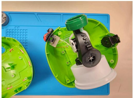
2. Lift out the lady bug switch and set aside. Remove the one screw holding the switch attached a small circuit board in place and flip it over to see where the yellow wire connects to the 3rd connection from the left. This is the wire you will cut to modify the toy. Cut this wire about an inch from the circuit board and strip both new ends of the yellow wire.
