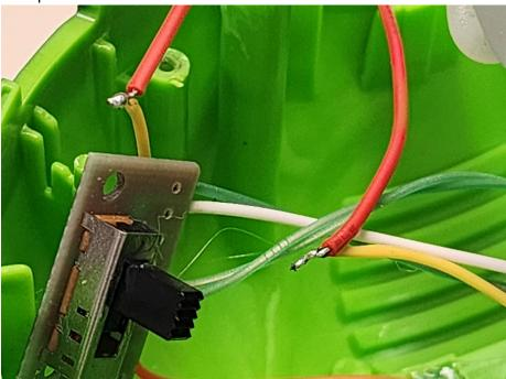
5. Protect the 2 solder joints with either shrink tube or electrical tape.
