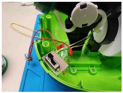
6. Drill a ¼" hole in the back of the toy at the location shown in the picture below. Insert the switch jack and hold it in place with the nut. Use needle nose pliers to ensure it is tight.
