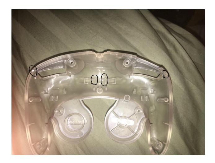
On the top shell, there is just one small post that needs to be removed, circled in the image below. This must be removed if you plan to use OEM parts in the shell.
