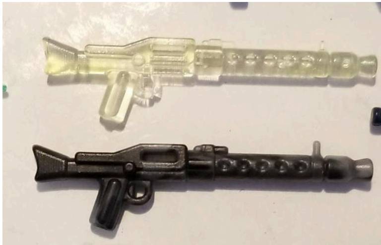
-Minigun Proto (Barrel and receiver were one piece that was a pain to inject)
