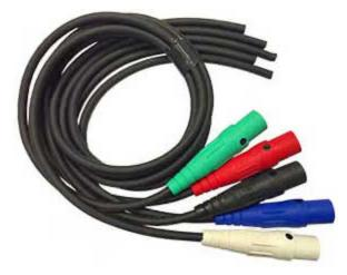
• Banded 5-wire feeder cables, male camlock x female camlock, 100A 240V, 50 FT LG. These are the main three-phase cables that connect the generator to the power pagodas. Since each of the 5 wires have individual connectors, it is easy to connect them wrong, so you will need to pay close attention to the wire colors at both ends of the cable. We use QTY 2.
