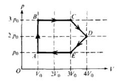
An ideal gas undergoes a cyclic process as shown on the graph above of pressure *p* versus volume V.
