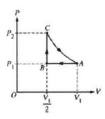
2004Bb5 One mole of an ideal gas is initially at pressure  $P_1$ , volume  $V_1$ , and temperature  $T_1$ , represented by point A on the PV diagram above. The gas is taken around cycle ABCA shown. Process AB is isobaric, process BC is isochoric, and process CA is isothermal.
