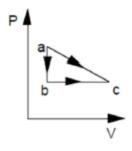
A gas can be taken from state a to c by two different reversible processes,  $a \Rightarrow c$  or  $a \Rightarrow b \Rightarrow c$ . During the direct process  $a \Rightarrow c$ , 20.0 J of work are done by the system and 30.0 J of heat are added to the system. During the process  $a \Rightarrow b \Rightarrow c$ , 25.0 J of heat are added to the system. How much work is done by the system during  $a \Rightarrow b \Rightarrow c$ ? (A) 5.0 J (B) 10.0 J (C) 15.0 J (D) 20.0 J
