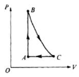
10. Gas in a chamber passes through the cycle ABCA as shown in the diagram above. In the process AB, 12 joules of heat is transferred to the gas. In the process BC, no heat is exchanged with the gas. For the complete cycle ABCA, the work done by the gas is 8 joules. How much heat is added to or removed from the gas during process CA?
