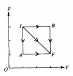
6. If three identical samples of an ideal gas are taken from initial state I to final state F along the paths IAF, IF, and IBF as shown in the P-V-diagram above, which of the following must be true?
