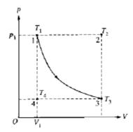
16. **Multiple Correct.** An ideal gas is initially in a state that corresponds to point 1 on the graph above, where it has pressure  $p_I$ , volume  $V_I$ , and temperature  $T_I$ . The gas undergoes an isothermal process represented by the curve shown, which takes it to a final state 3 at temperature  $T_3$ . If  $T_2$  and  $T_4$  are the temperatures the gas would have at points 2 and 4, respectively, which of the following relationships is true? Select two answers:
