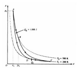
1983B4. The pV-diagram above represents the states of an ideal gas during one cycle of operation of a reversible heat engine. The cycle consists of the following four processes.
