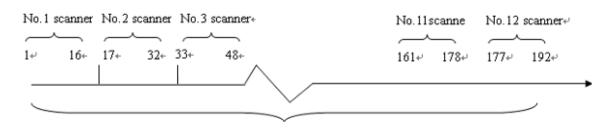
12 scanners, each is assigned 16 channels.
