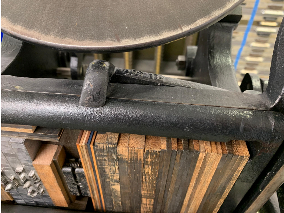
The hook is properly set on the forme. The forme should be tight against the steel back of the press
