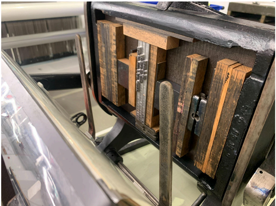
The metal grippers are the long rods sticking up. Make sure these will not come into contact with any type or high points of the forme.
