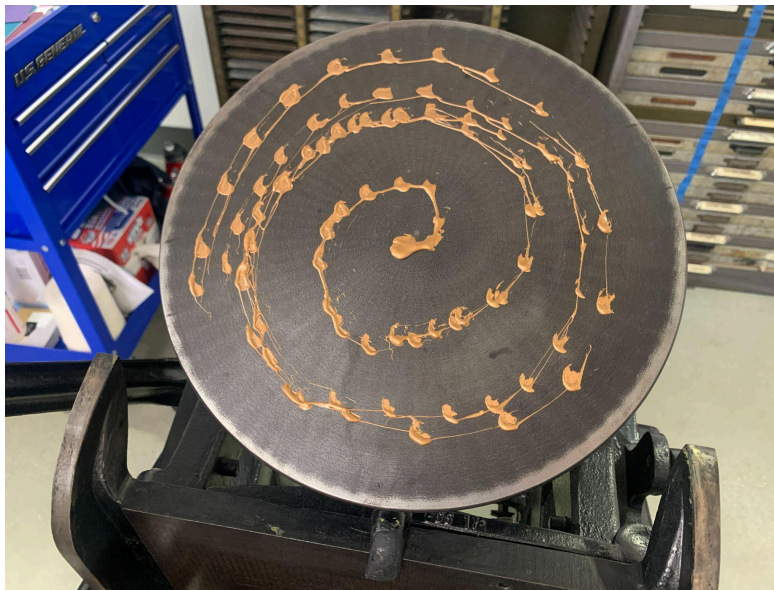
Ink dotted in a spiral pattern to help spread the ink on the inking disk
