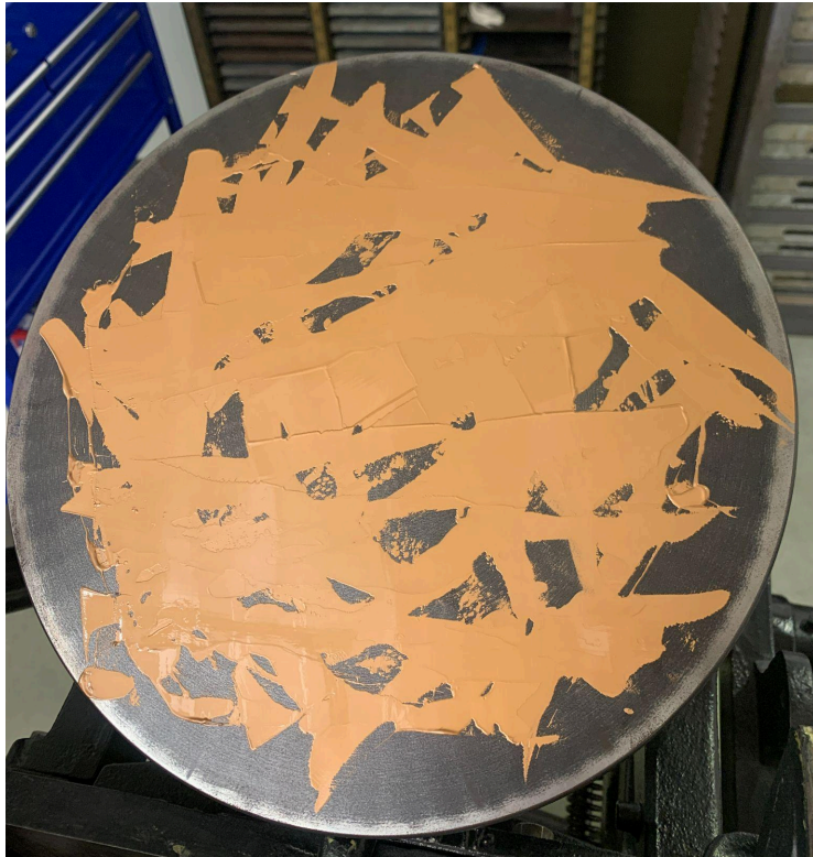
Ink after being spread with the inking knife. Make sure not to scratch the surface of the disk with the corners of the inking knife.
